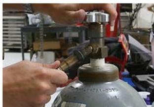
**1** Sensors were tested using laboratory gas specifically formulated to yield 11.76 AFR and 13.15 AFR. This way each sensor sees the exact same "exhaust gas", letting us measure the accuracy and responsiveness of each
