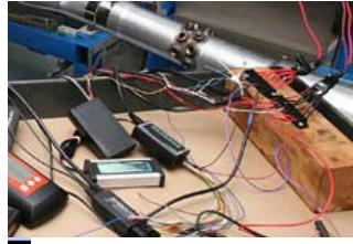
**3** Nine bungs were welded into the exhaust; eight for the sensors under test and one for Westech's own meter. Datalogging was performed during the engine run-in to assess the capabilities of each meter.
