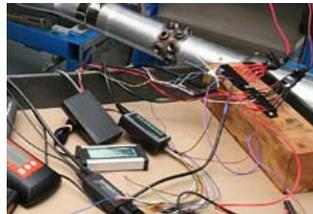
**4** A common power and ground supplied each meter to ensure no other variables influenced the testing.
