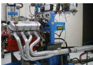
**2** After testing with lab gas the sensors were run-in for an hour with race fuel, on a test engine (Westech just happened to have a Chevy motor in the dyno room that day.) The run in simulates the wear and tear a sensor
